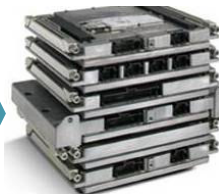
PC104+ Stack with Thermal Plates (no moving parts)
